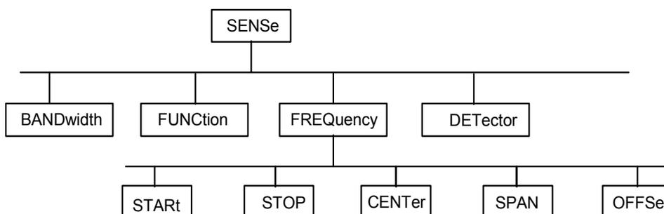
Fig. 5.1 Tree structure the SCPI command systems using the SENSe system by way of example
