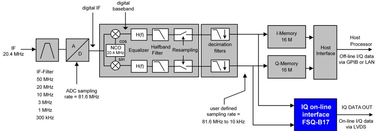
**Fig. 4.18** Block diagram of the IQ downconverter
