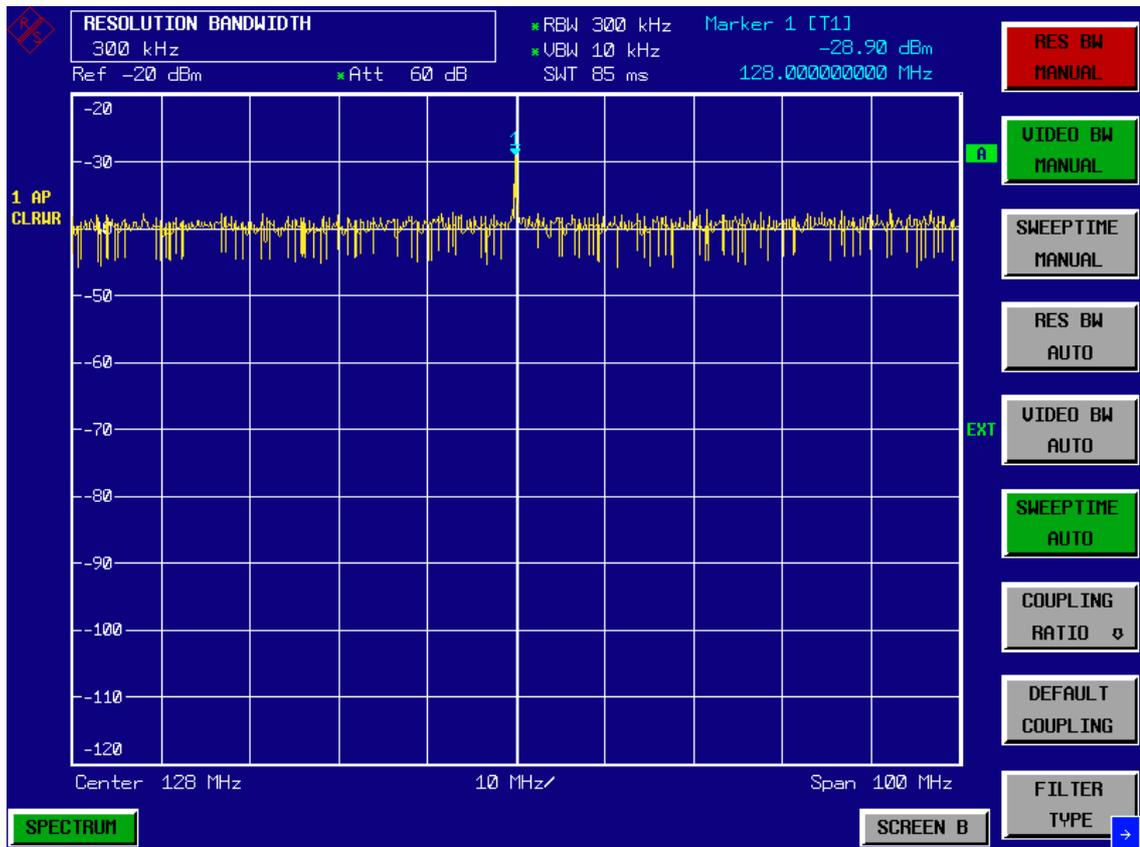
Fig. 2.12 Reference signal at a smaller resolution bandwidth
