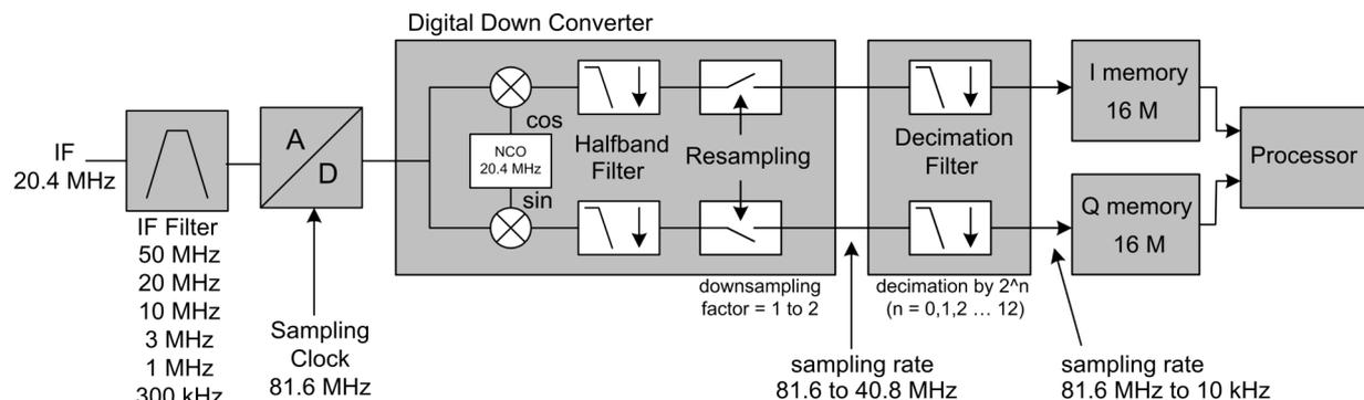
Fig. 6.1 Block diagram illustrating the R&S FSQ signal processing
