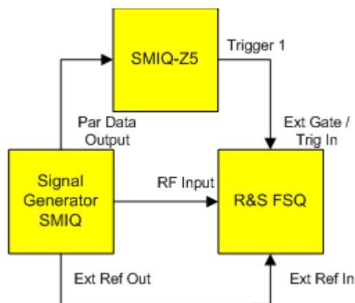
The R&S SMIQ has to be equipped with options R&S SMIQ-B10 or R&S SMIQ-B20 (modulation coder) and R&S SMIQ-B11 (data generator).
