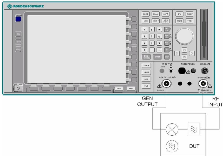
Fig. 4.26 Test setup for frequency converting measurements
