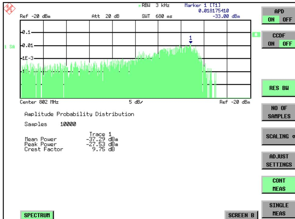
**Fig. 4.12 Display of the amplitude probability distribution**
