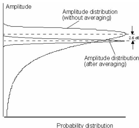
This low average value is usually corrected in noise power measurements by a 2.5 dB factor. Therefore the R&S FSQ offers the selection of linear averaging. The trace data are delogarithmized prior to averaging, then averaged and logarithmized again for display on the screen. The average value is always correctly displayed irrespective of the signal characteristic.
