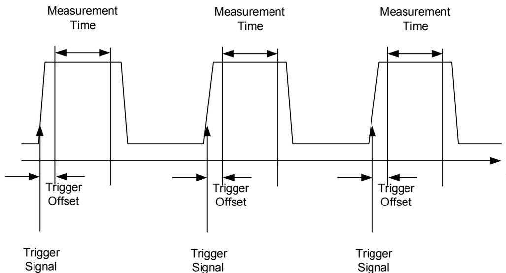
Depending on the settings made, the measurements are performed with the RMS detector for RMS power or the PEAK detector for peak power. For all these measurements, TRACE 1 of the selected system is used.
