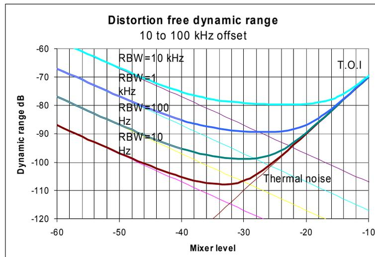
**Fig. 2.6** Intermodulation-free dynamic range of the R&S FSQ as a function of level at the input mixer and of the selected resolution bandwidth (useful signal offset = 10 to 100 kHz, DANL = -157 dBm /Hz, TOI = 25 dBm; typical values at 2 GHz).
