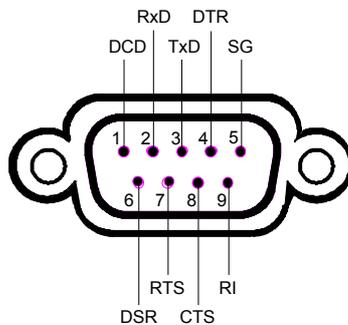
Fig. 8.4 Pin assignment of the RS-232-C interface
