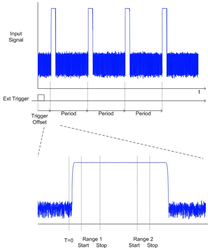
The gate ranges define the part of the I/Q capture data taken into account for the statistics calculation.
