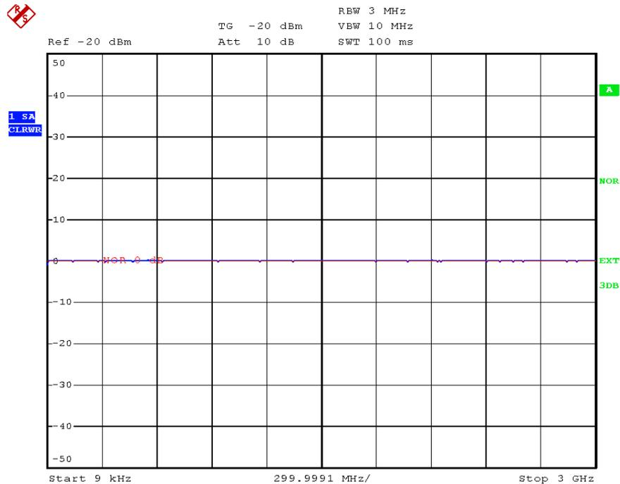
**Fig. 4.31 Normalized measurement, shifted with REF VALUE POSITION 50%**
