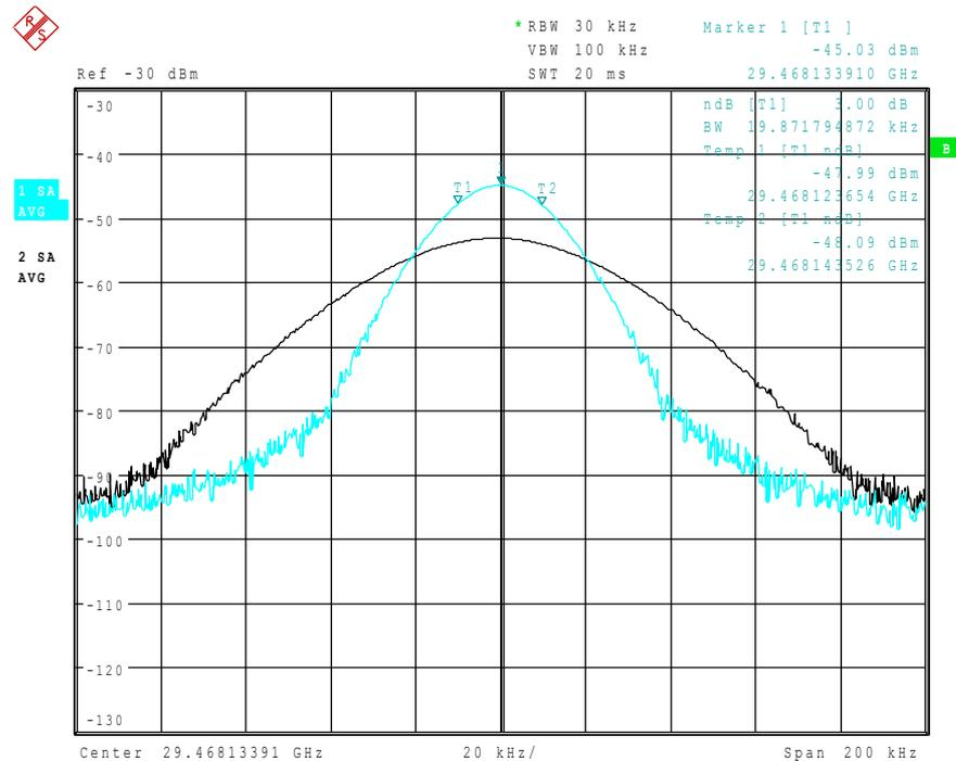
**Fig. 4.39** Different mixer products represented at the same frequency in the test sweep and reference sweep
