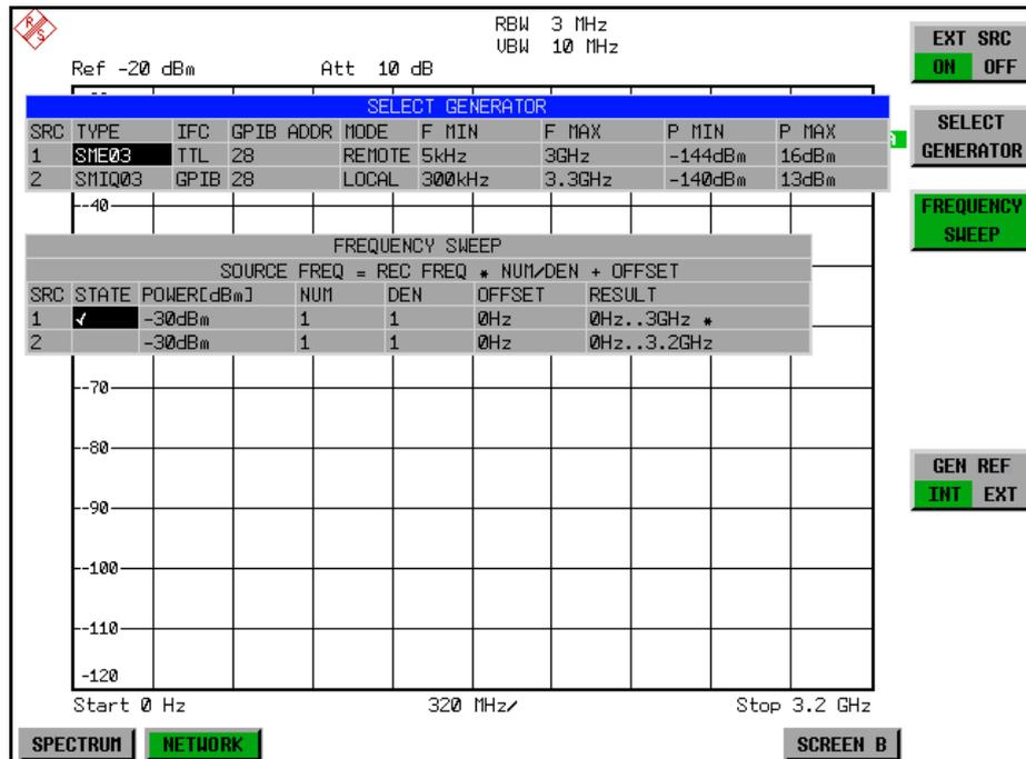
The *EXT SOURCE* softkey opens a submenu for configuration of the external generator.
