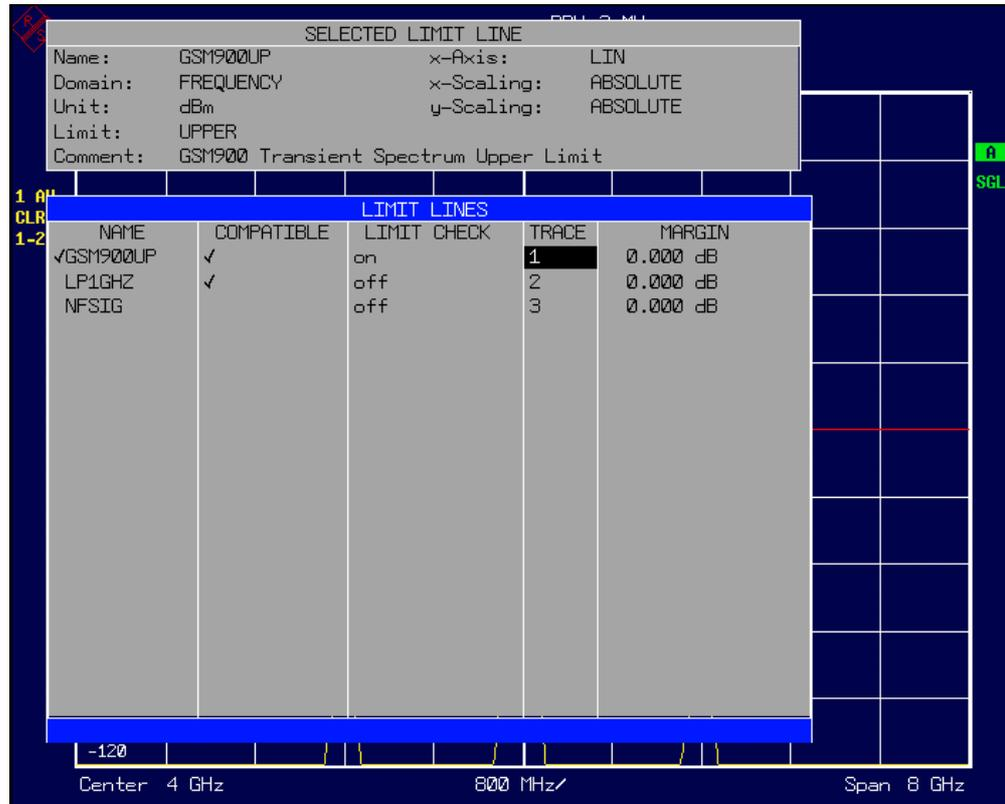
The *SELECTED LIMIT LINE* display field provides information concerning the characteristics of the marked limit lines.
