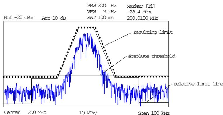
The preset value is at -200 dBm. The field is displayed if the value RELATIVE is entered in the field Y-SCALING.
