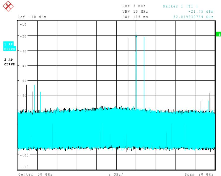
The reference sweep is performed using a LO setting shifted downwards by  $2 \cdot \text{IF} / \text{Harmonic\#}$ . Input signals in the wanted sideband that are converted by means of the set harmonic are displayed in both traces at the same position on the frequency axis. Image signals and mixer products caused by other harmonics are displayed in both traces at different positions.
