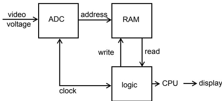
**Fig. 4.11 Simplified block diagram for APD measurement**
