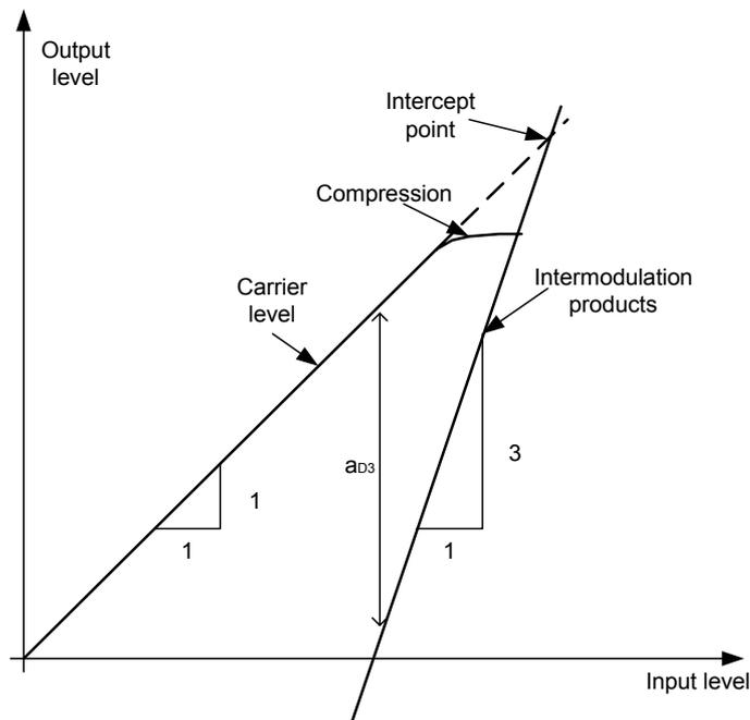
**Fig. 2.2** Level of the 3<sup>rd</sup> order intermodulation products as a function of the level of the useful signals
