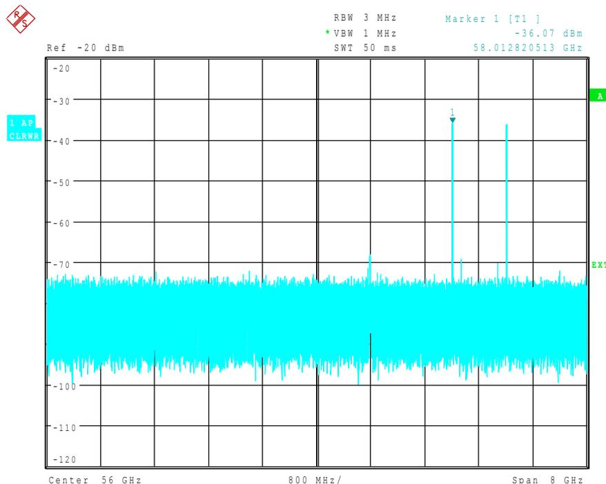
Fig. 4.41 Spectrum at the multiplier output recorded with an external mixer
