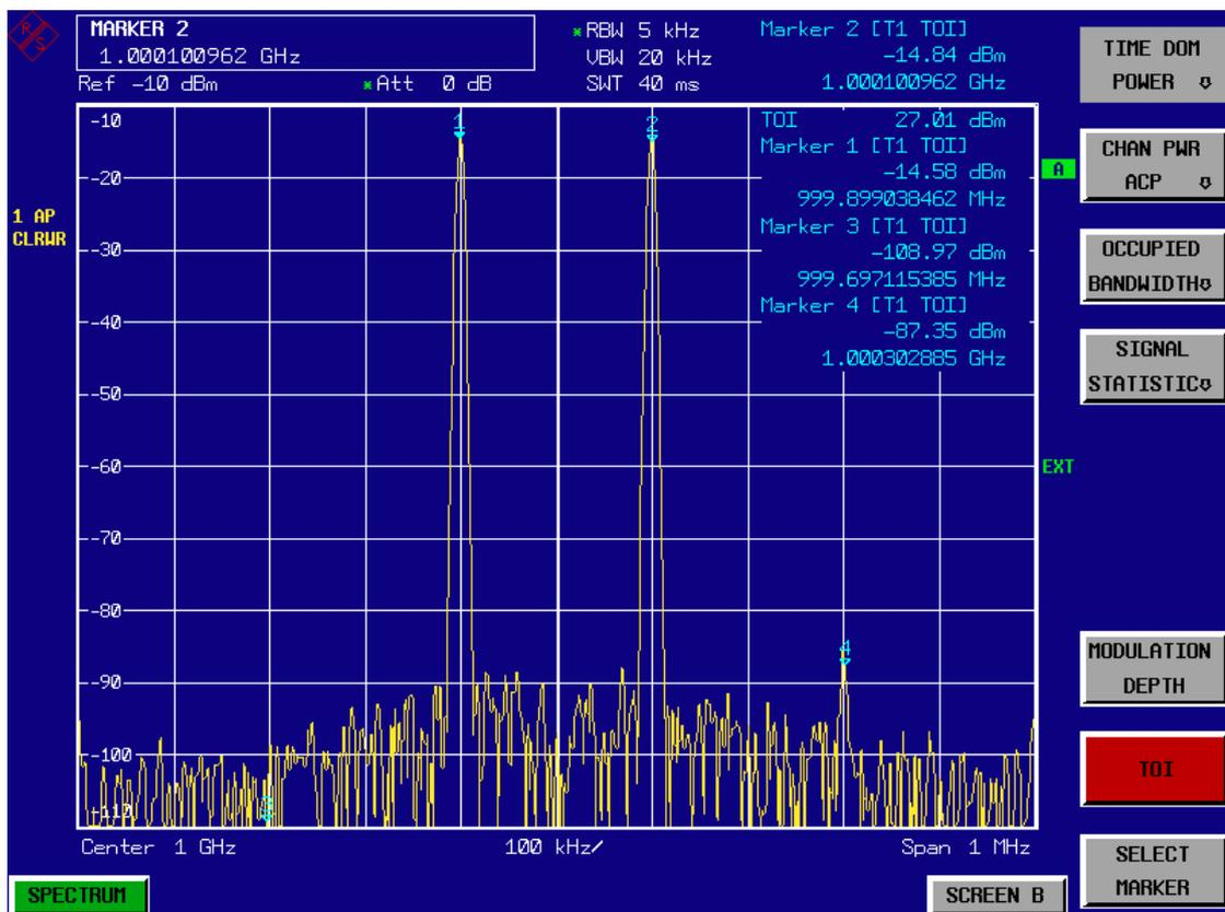
**Fig. 2.3** Result of intrinsic intermodulation measurement on the R&S FSQ. The 3<sup>rd</sup> order intercept (TOI) is displayed at the top right corner of the grid
