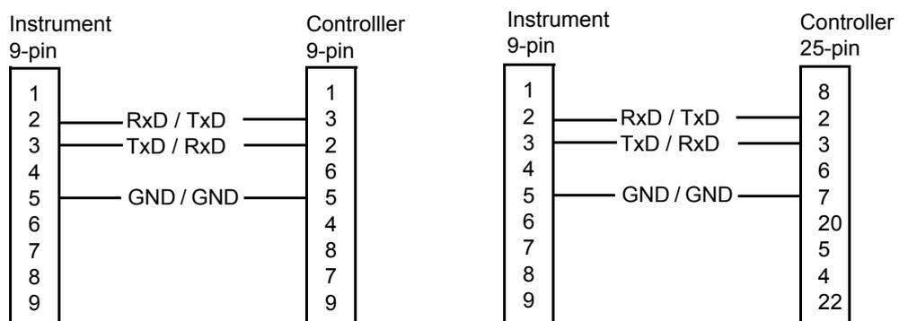
Fig. 8.5 Wiring of the data lines for software handshake
