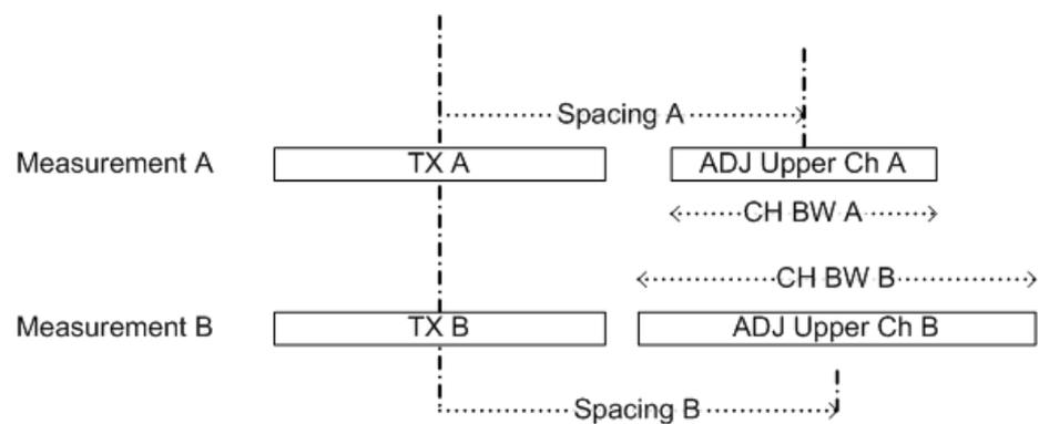
ACP Measurement A and Measurement B are using identical TX channel settings (Channel Bandwidth).
