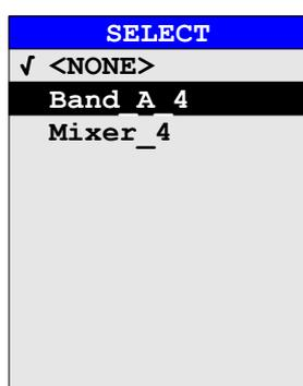
After selection of a file the parameters *BIAS* for the *SELECT BAND* table are taken from that file. The selected mixer type must correspond to the file entry *PORTS*. It is not possible to modify these parameters during operation.
