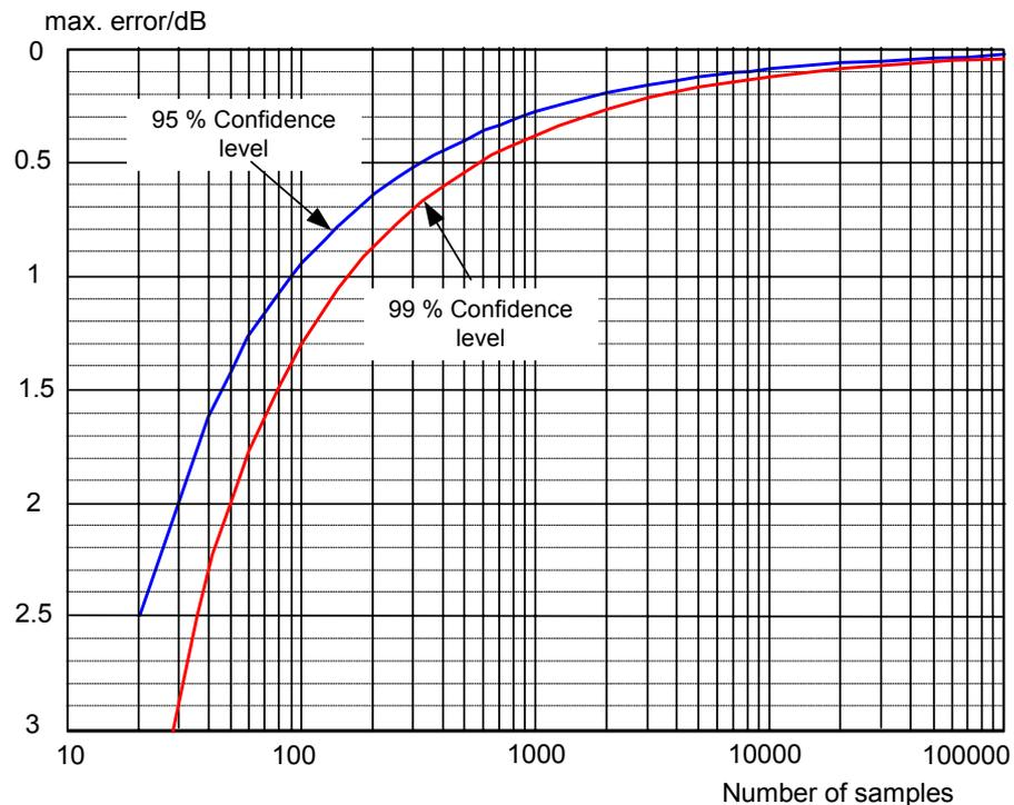
**Fig. 2.16 Repeatability of channel power measurements as a function of the number of samples used for power calculation**
