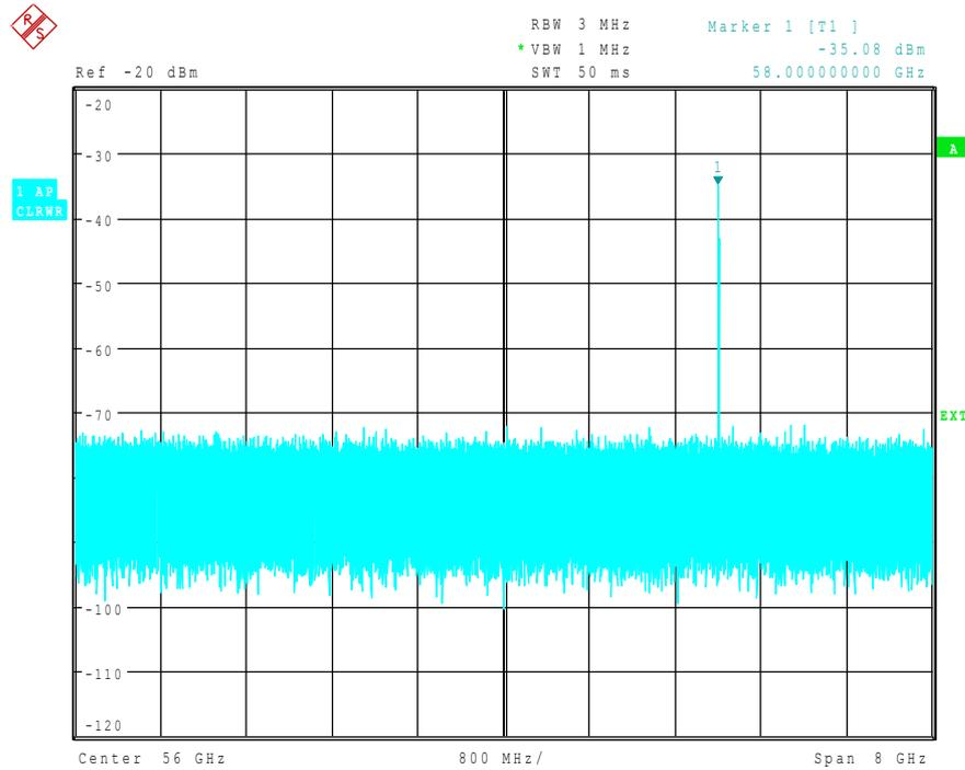
**Fig. 4.42** Output spectrum of the multiplier recorded with an external mixer and AUTO ID
