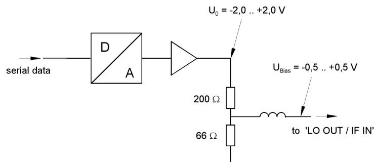
Fig. 4.36 Bias circuit of the R&S FSQ
