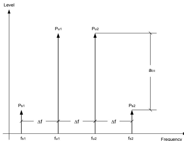
**Fig. 2.1** 3<sup>rd</sup> order intermodulation products
