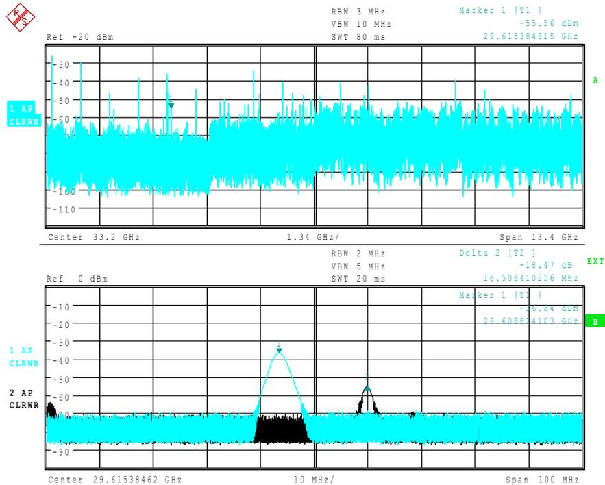
**Fig. 4.38** Screen A: Unwanted mixer product not detected by *AUTO ID*
