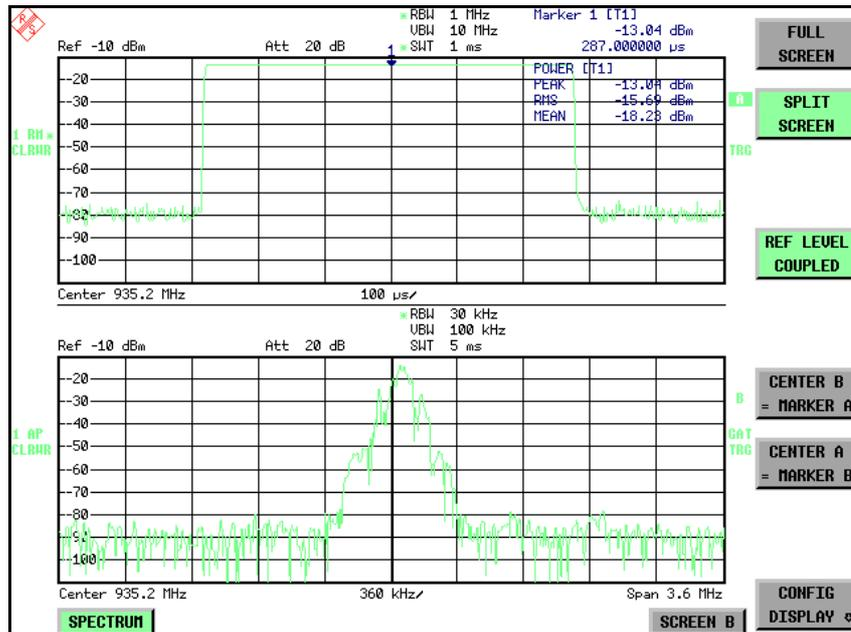
Fig. 4.16 Typical split-screen display, settings are uncoupled
