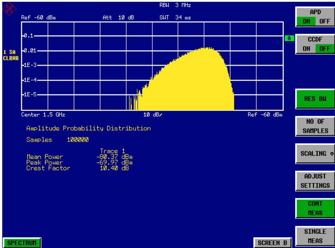
Fig. 2.35 Amplitude probability distribution of white noise
