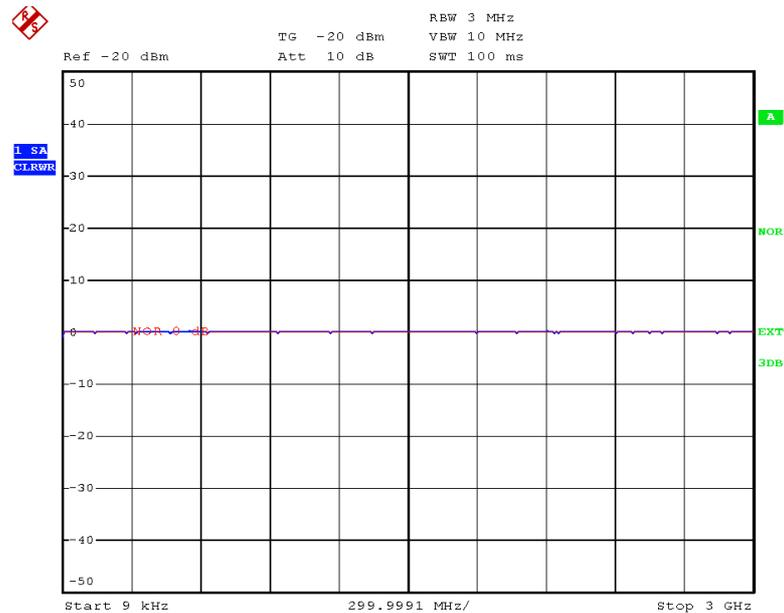
Fig. 4.22 Normalized measurement, shifted with REF VALUE POSITION 50%
