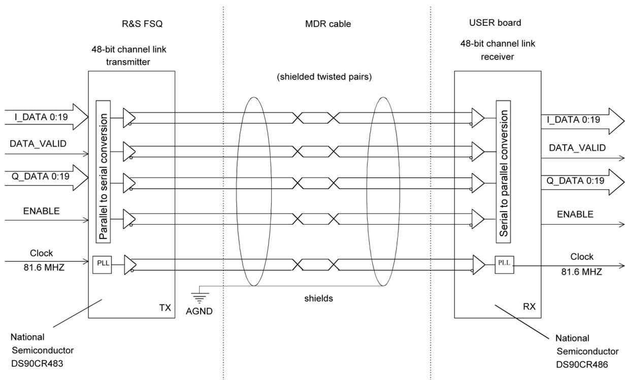
Fig. 4.19 R&S FSQ LVDS interface connection overview
