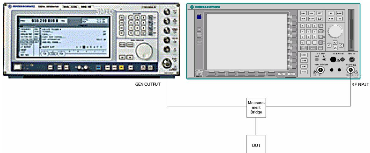
*Fig. 4.34 Test setup for reflection measurement*
